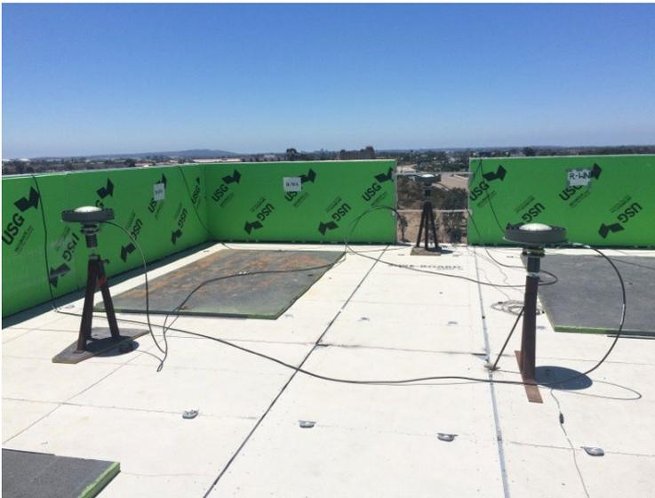
Figure 10: Roof antennas mounted on new 2' stands. Left: Roof South, Center: Roof West, Right: Roof Center.
