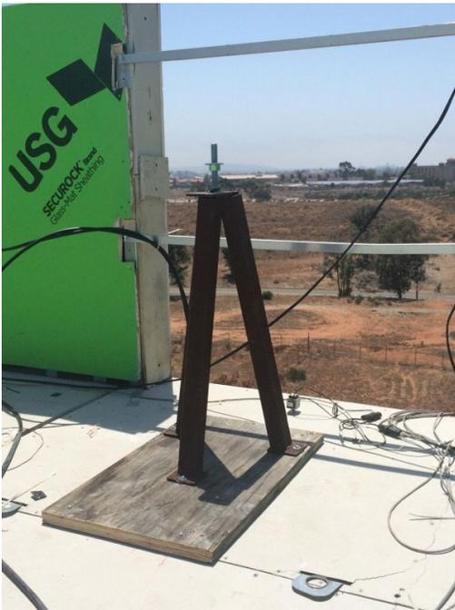
Figure 8: The new 2' mount at the western edge of the roof, installed for the final day of seismic tests.
