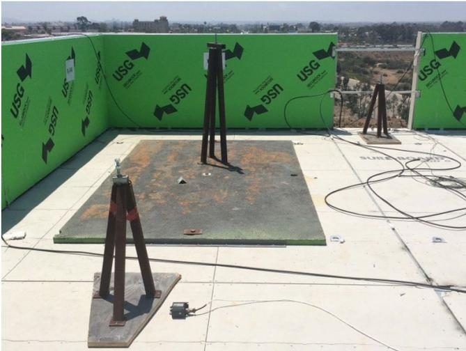
Figure 9: New 2' stands installed on the roof for the final day of seismic tests. Left: Mount for station Roof South. Center: Removed roof SW mount. Right: Mount for station Roof West.
