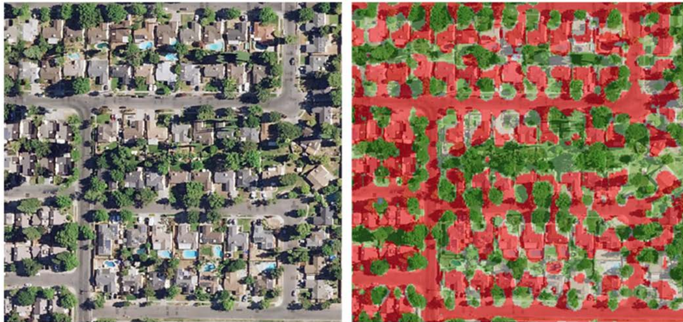
Figure 8 Original Image and label image. Left image show high resolution aerial image and right one shows label data overlain on aerial image with transparency 50%. The color red and green represent impervious surface and trees respectively. Whole classes are listed in Table 3.
