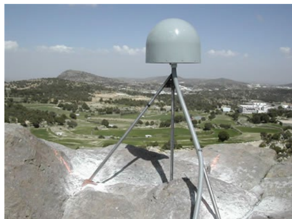
Figure A.1. Two types of geodetic monuments (Top) deeply-anchored drill-braced designed by D. Agnew and F. Wyatt; (Bottom) Short-braced in bedrock.
